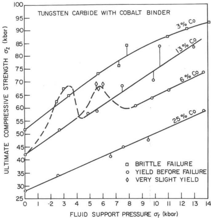
Fig. 3 Variation of ultimate compressive strength as a function of fluid support pressure for tungsten-carbide materials with cobalt binder
